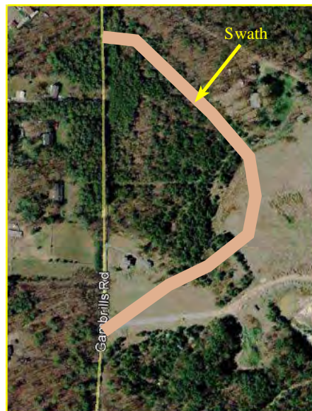
Initially Clear Swath for Earth Berm, Silt Fence, Trap & Other Perimeter Controls
